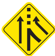
Free flow (added lane)
